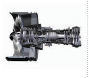
A cutaway of the geared turbofan engine being developed by Pratt & Whitney
